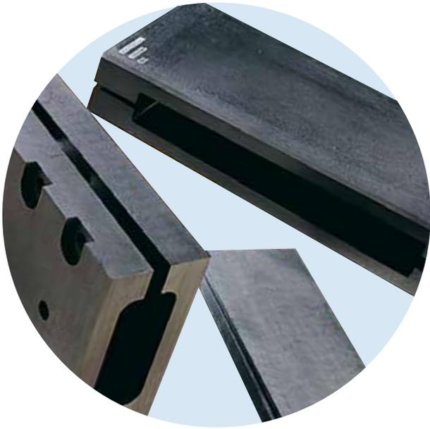
... depends mainly on the composition of the alloy to be cast: grey iron requires a graphite resistant to wear abrasion; brass, a graphite relatively dense but with enough open porosity to allow zinc to evaporate in the area of the solidification front; non-ferrous alloys containing elements like nickel or cobalt need high density graphite to reduce chemical attack of the graphite die...
